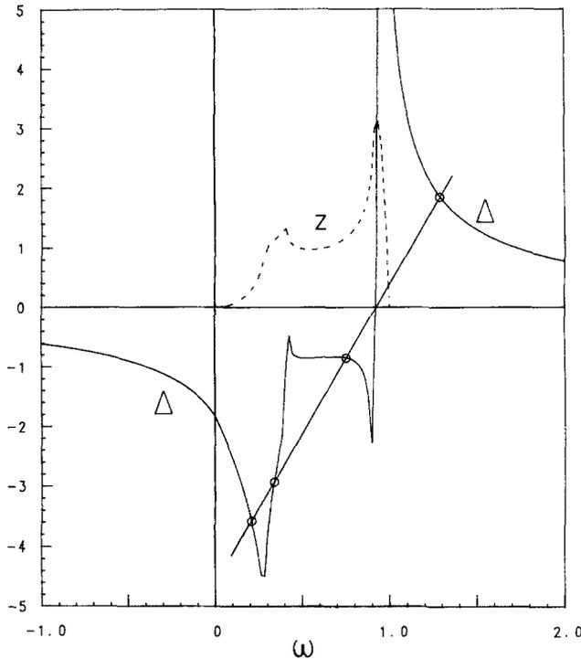
**Fig. 1.** The model phonon density of states  $Z(\omega)$  adopted is displayed together with the corresponding  $\Delta(\omega)$ , defined in (3.13). Solutions of (4.1) are indicated for  $\omega_0=0.921$ ,  $\omega_r=1.3$  and  $g^2=0.2$ ; the maximum  $g^2=0.348$ . Energies are measured in units of the maximum phonon energy
