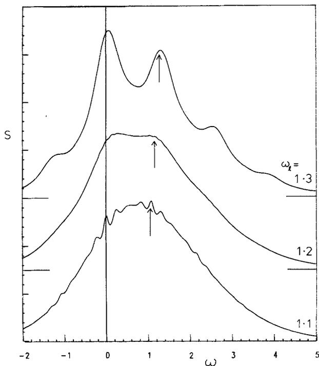
Fig. 8. The  $g^2$  variation of  $S(k, \omega)$  for fixed  $\omega_0$  is illustrated for  $\omega_0 = 0.7$ ,  $k^2/2M = T = 1$ . The base lines are shifted for clarity. The values of  $\omega_r$  are:  $g^2 = 0.107$ ,  $\omega_r = 1.1$ ;  $g^2 = 0.200$ ,  $\omega_r = 1.2$ ;  $g^2 = 0.313$ ,  $\omega_r = 1.3$
