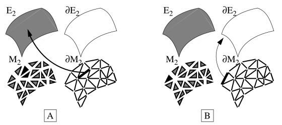
**Figure 1**: In a compatible mesh, for each edge, either A: the edge is part of the surface and has two neighboring faces, or B: the edge is part of the boundary of the surface and has one neighboring face.
