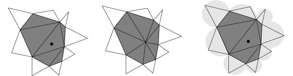
**Figure 5**: Bowyer's algorithm for Delaunay mesh refinement. Left: The original mesh with a new node about to be added and the influence domain of the new node. Middle: the structure in the influence domain replaced by radial elements from the new node, Right: the region where another node may not be added in parallel
