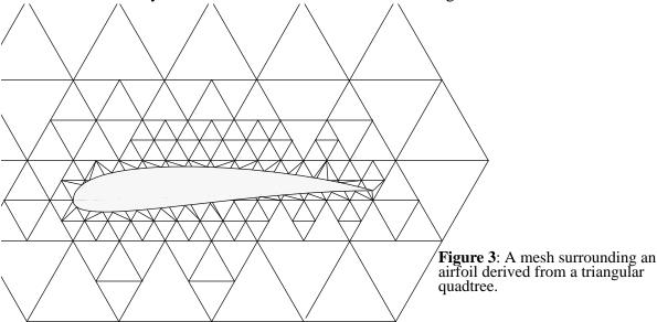
The problem with this approach to mesh creation is that in many applications, such as CFD, the quality of the solution depends critically on the correct treatment of boundaries, which is where the mesh of Figure 3 has particularly badly shaped elements. While there are curative methods to improve the mesh, the essential problem is that the mesh is distorted to fit the boundaries, rather than first laying out the boundaries and creating the mesh to accommodate them.
