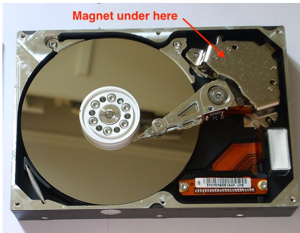
Figure 10-1 How to extract the powerful magnet from a hard disk drive (Wikimedia Alessio Sbarbaro)
